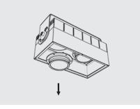
3. Disconnect cables attached to LED module and unfasten screws to remove LED module for replacement.
