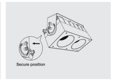
3. Rotate fixture to desired angle and secure position by fastening M10 screws onto the curved slot.
