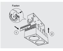
2. Insert side cover plates and fixture, fasten M10 screw onto the middle of mounting bracket on each side.
