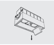
2. Disconnect cables attached to LED driver and unscrew bracket to remove LED driver for replacement.
