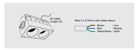
4. Connect AC cables to incoming power supply. Installation complete.
