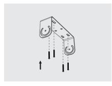
1. Secure mounting bracket onto intended mounting surface (mounting screws not included).
